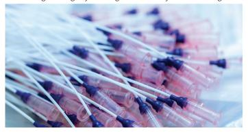
Resins with different properties are combined in a single part often to improve functionality, product differentiation, aesthetic appeal, or marketability over traditional designs. The process is commonly referred to as two-shot, 2K or 2C molding and often involves the combination of hard thermoplastics and a soft thermoplastic elastomer (TPE). In some applications the material properties of TPEs are not sufficient so thermoplastics are utilized alongside a silicone elastomer.
