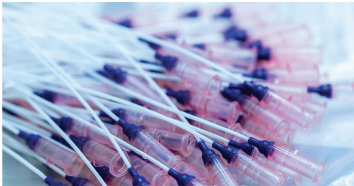
Resins with different properties are combined in a single part often to improve functionality, product differentiation, aesthetic appeal, or marketability over traditional designs. The process is commonly referred to as two-shot, 2K or 2C molding and often involves the combination of hard thermoplastics and a soft thermoplastic elastomer (TPE). In some applications the material properties of TPEs are not sufficient so thermoplastics are utilized alongside a silicone elastomer.
